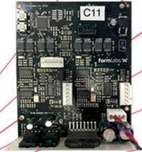
FORMLABS FORM 1 GALVO MOTORS DRIVER
